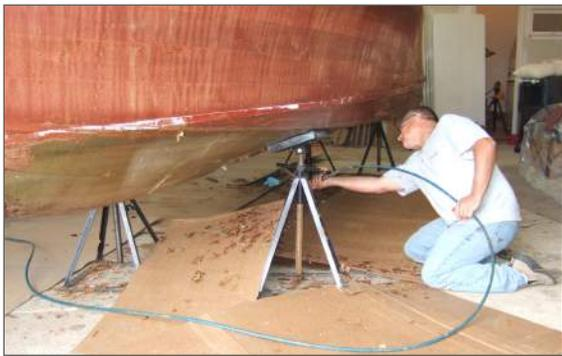
The stripper was applied to the bottom in less than 10 minutes with no wasted stripper. After 3 hours of dwell time, the bottom was scraped in 1.5 hours.
