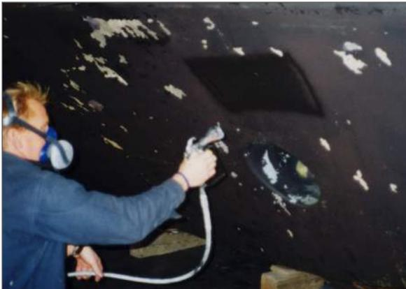
Spraying "Phase 1 Paste" on starboard side above the bow thruster.
