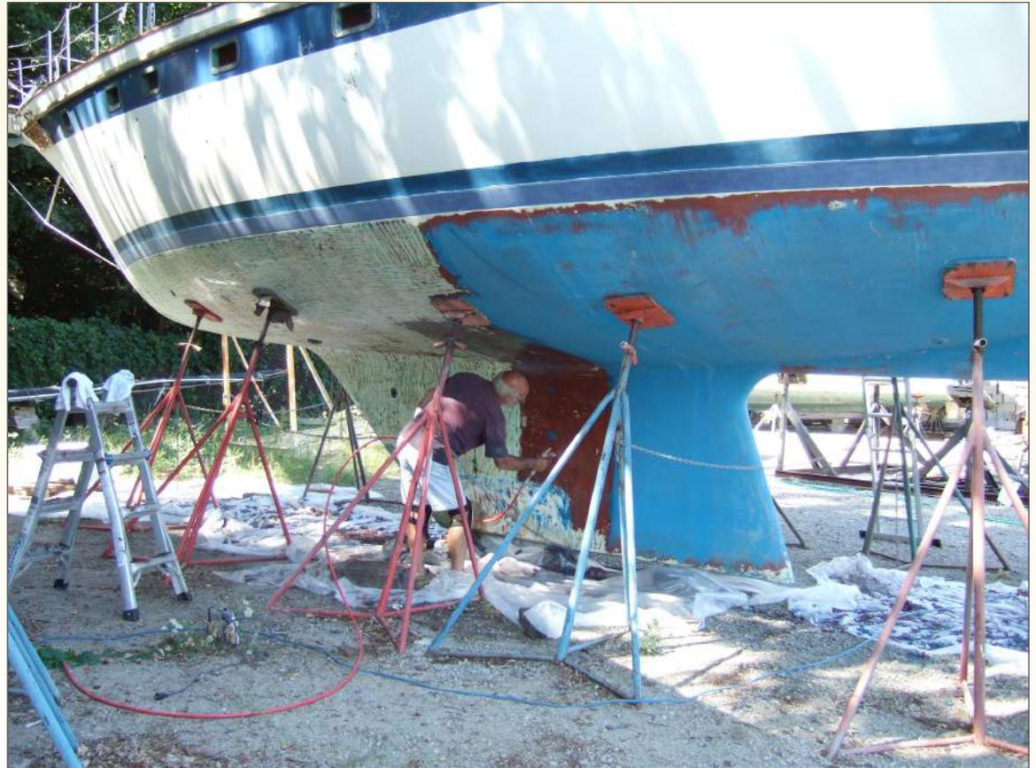
Formosa 47 - The owner applied the Star 10 "Phase 1 Paste", allowed the product to "dwell" and then scraped off the ablative primer coat and the ablative top coat at the same time on one side, in one day.
